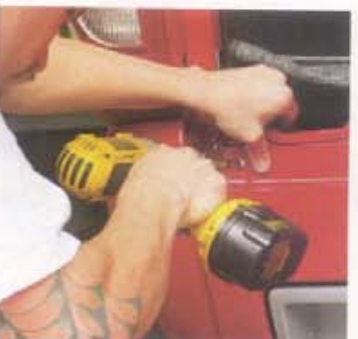
15. Here, David installed the screws using a drill to properly mount the roll pan.
