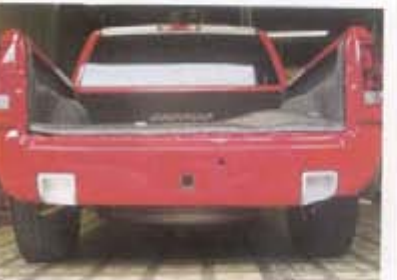
16. Before the tailgate was installed, this is what the new roll pan looked like.
