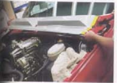
11. Next up, the guys installed the Street Scene wiper cowl.
