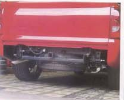
12. The Street Scene Silverado was already equipped with a hidden hitch, and fortunately for us, Street Scene makes a roll pan just for that application.
