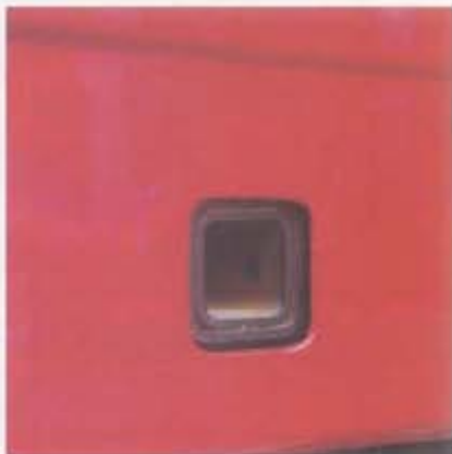
17. Fitting like a well-formed glove, the new Street Scene roll pan fit around the hitch receiver perfectly.
