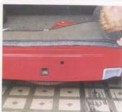
13. Colby and David placed the new roll pan into place and performed a quick fitment test.
