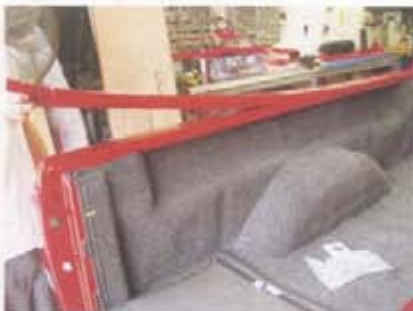
20. Simpler than turning the key, the Smooth Bed Caps simply lay flat on the bedrails and are secured by 3M double-sided tape.
