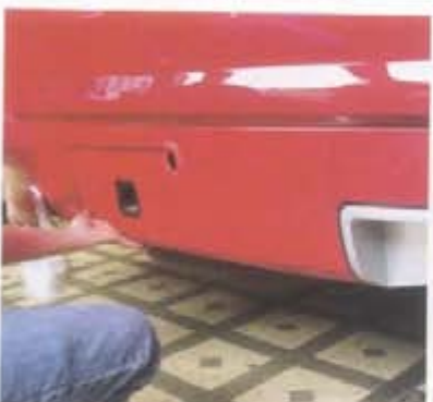
14. While Colby held the roll pan in place, David marked where the new mounting screws would be needed to secure the pan with a punch.
