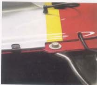
9. After everyone was satisfied with the fitment, special retaining clips were installed to lock the wiper cowl into place.
